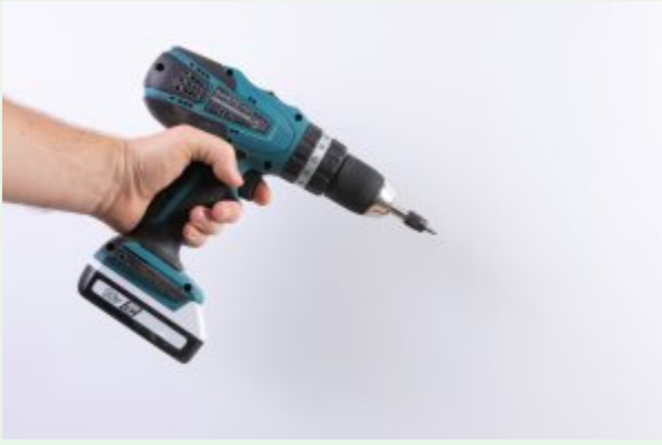
Figure 11.3: The 'trigger' on the hand drill is a small-scale dead man's switch
