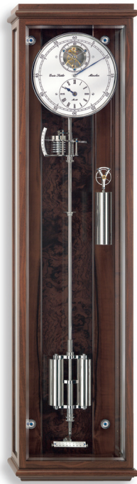
FIGURE 136 A precision second pendulum, thus about 1 m in length; almost at the upper end, the vacuum chamber that compensates for changes in atmospheric pressure; towards the lower end, the wide construction that compensates for temperature variations of pendulum length; at the very bottom, the screw that compensates for local variations of the gravitational acceleration, giving a final precision of about 1 s per month (© Erwin Sattler OHG).
