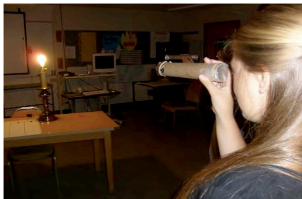
FIG. 1.11 Looking at a light bulb through a pinhole camera made out of a paper towel roll.
