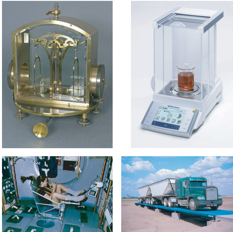
FIGURE 71 Mass measurement devices: a vacuum balance used in 1890 by Dmitriy Ivanovich Mendeleev, a modern laboratory balance, a device to measure the mass of a cosmonaut in space and a truck scales (© Thinktank Trust, Mettler-Toledo, NASA, Anonymous).
