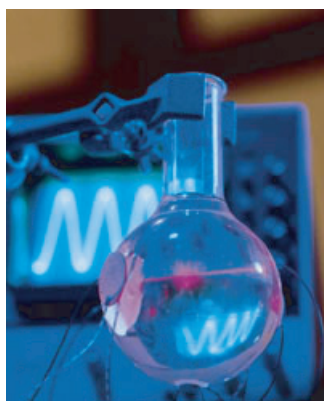
FIGURE 63 Observation of sonoluminescence with a simple set-up that focuses ultrasound in water (© Detlef Lohse).
