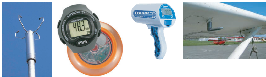
FIGURE 16 Some speed measurement devices: an anemometer, a tachymeter for inline skates, a sports radar gun and a Pitot–Prandtl tube in an aeroplane (© Fachhochschule Koblenz, Silva, Tracer, Wikimedia).
