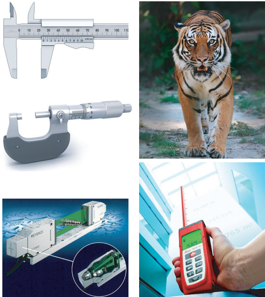
FIGURE 23 Three mechanical (a vernier caliper, a micrometer screw, a moustache) and three optical (the eyes, a laser meter, a light curtain) length and distance measurement devices (© www.medien-werkstatt.de , Naples Zoo, Keyence, and Leica Geosystems).
