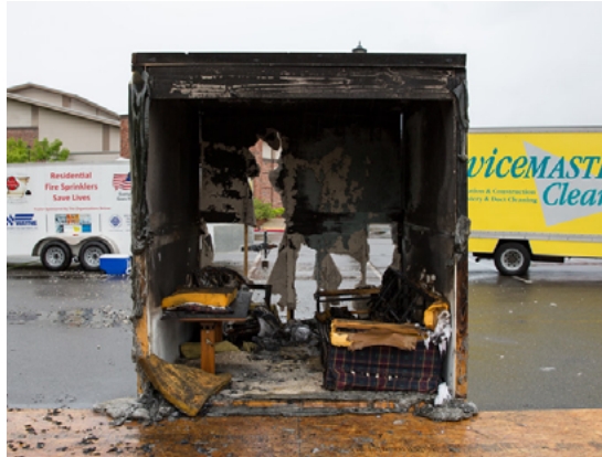
Fig.03/02 Fire sprinklers provide significant amount of protection, at a relatively reasonable cost. Especially for new construction, while lowering the fire resistance requirements for materials and assemblies.
