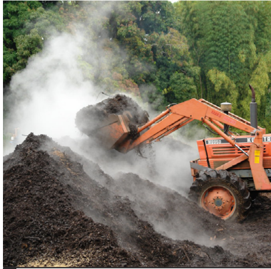
Fig.04/08 Compost mounds need to be frequently aerated, otherwise buried waste won't break down.
