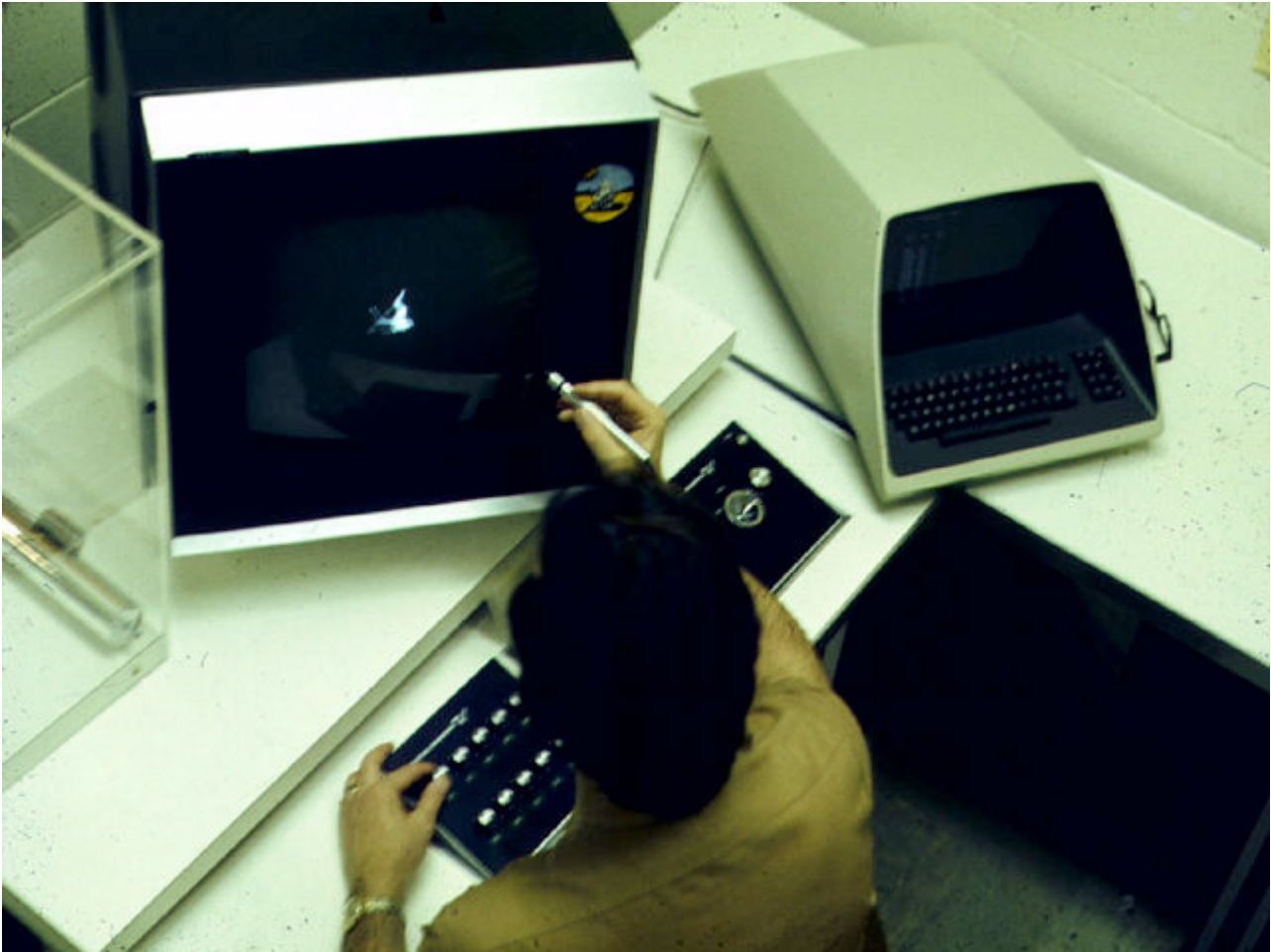
Chuck Csuri working with light pen attached to a Vector General vector graphics display
