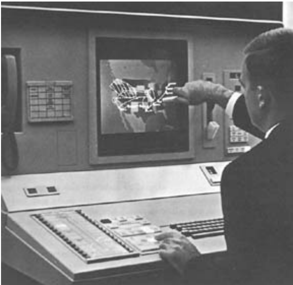
Bunker Ramo rear projection CRT
