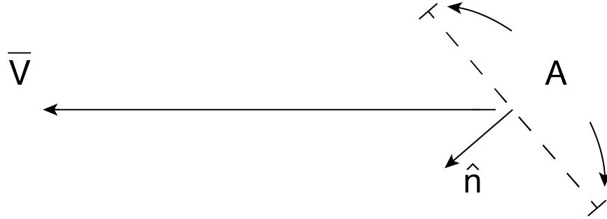
Fig 4.3 Flow through area A with outward normal \hat{\mathbf{n}} and velocity vector \bar{\mathbf{V}} .
