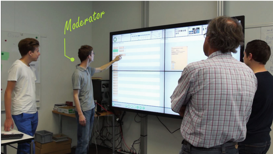
Fig. 1. aWall – digital Agile cardwall displayed on a large high resolution multi-touch wall ( 2 \times 2 46 Inch 4K displays) for planning and Agile team meetings.
