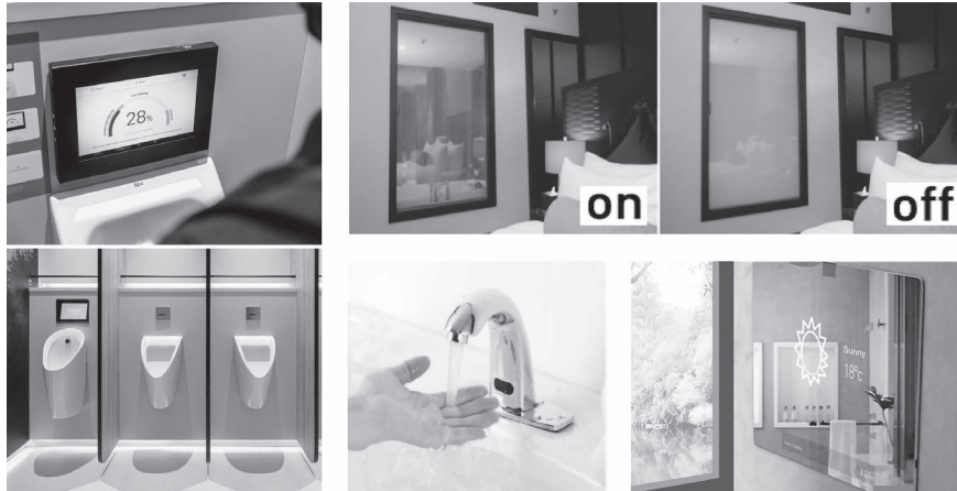
Figure 5.5 Above and below left: Intelligence urinal, which, through sensors, screens, and connections to analyse the data instantly, allows us to know the person’s hydration status instantly. Above right: Smart mirrors that turn opaque using facial biometric readings are useful for Alzheimer’s patients. Below right: Faucets with temperature and water flow sensors and smart mirrors with weather information.
