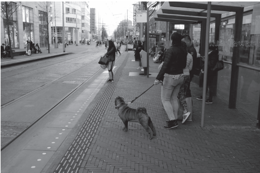
Figure 9.12a Show clear demarcation between tram lines, pedestrian waiting spaces, and tactile paving.
