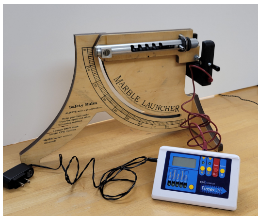
Figure 9.8: Experimental Initial Velocity of Marble Measured Using CPO Timer
