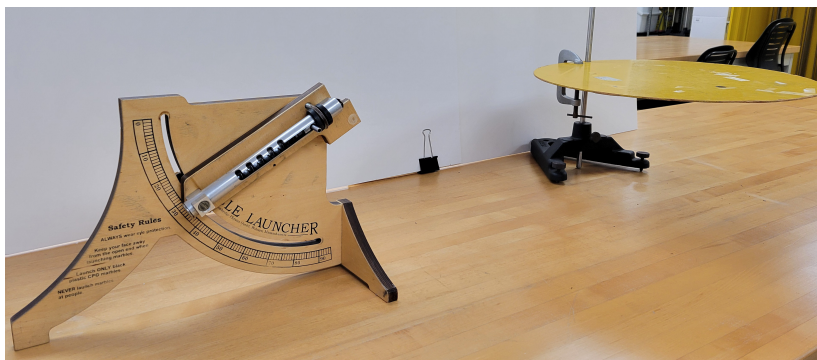
Figure 9.9: Measuring the Range of the Projectile Using a Landing Platform
