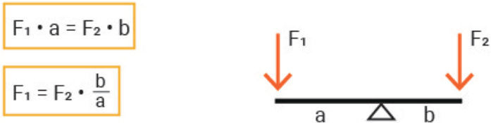
Figure 3-5: Archimedes' principle of the level
