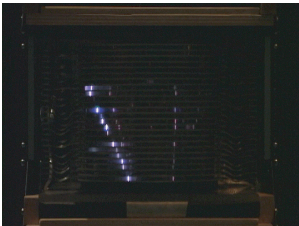
FIGURE 104 A modern spark chamber showing the cosmic rays that constantly arrive on Earth (QuickTime film © Wolfgang Rueckner).
