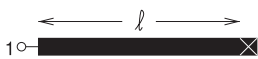
Figure 8-17: A 50 Ω shorted gold microstrip line with width w = 500 \mu\text{m} , length \ell = 1 \text{ cm} on a 600 μm thick alumina substrate with relative permittivity \epsilon_r = 9.8 and loss tangent \tan \delta = 0.001 .
