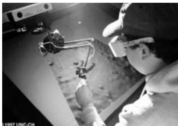
The GROPE force feedback system
