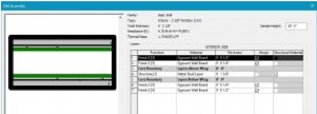
Figure 2.11 Basic Wall Interior – 3 1/8" Partition (1-hr)
