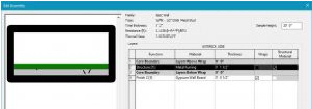
Figure 2.14 Basic Wall Soffit – ½” GWB Metal Stud
