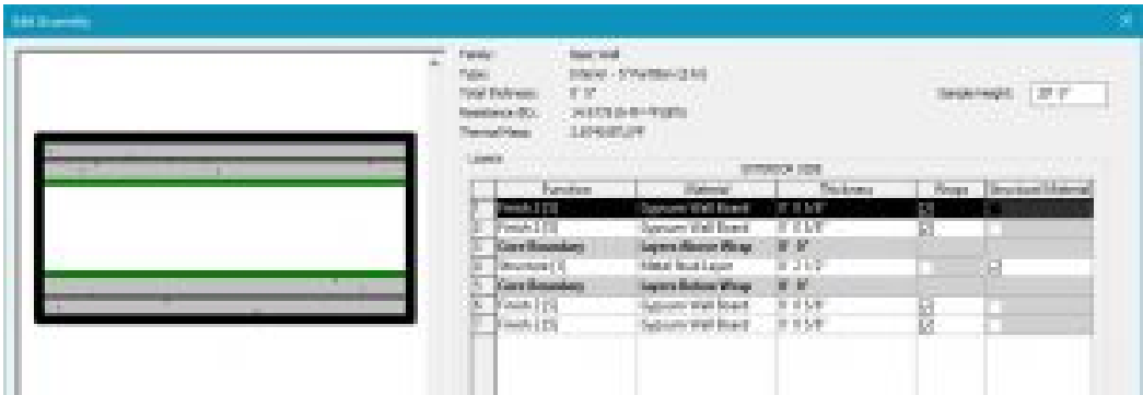
Figure 2.12 Basic Wall Interior – 5” Partition (2-hr)
