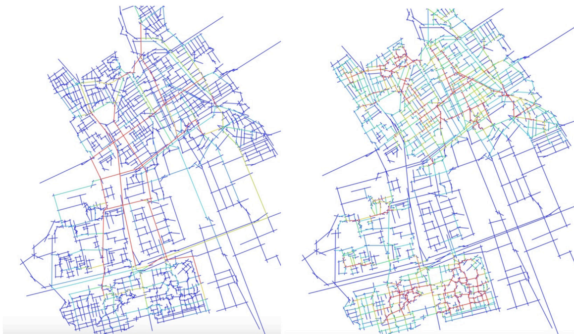
Figure 3: Angular choice analyses of Delft with a metrical radius of 5000 meters (left) and 500 meters (right). Maps by A. van Nes.
