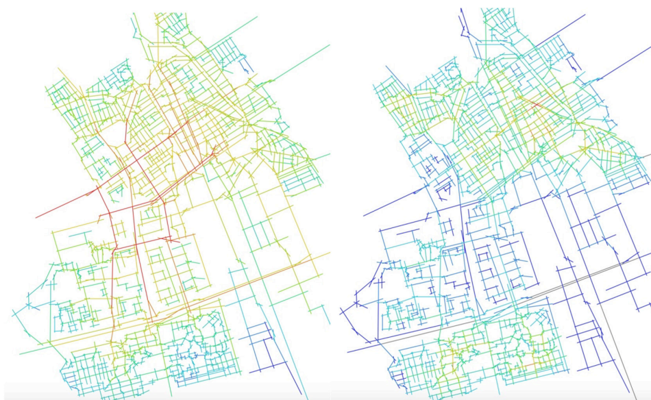
Figure 4: Segment integration analyses of Delft with a metrical radius of 5000 meters (left) and 500 meters (right).
