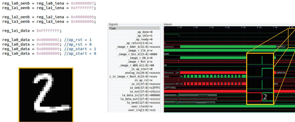
Figure 7. Testbench of the IC AI by AI implemented with SKY130A standard cells.
