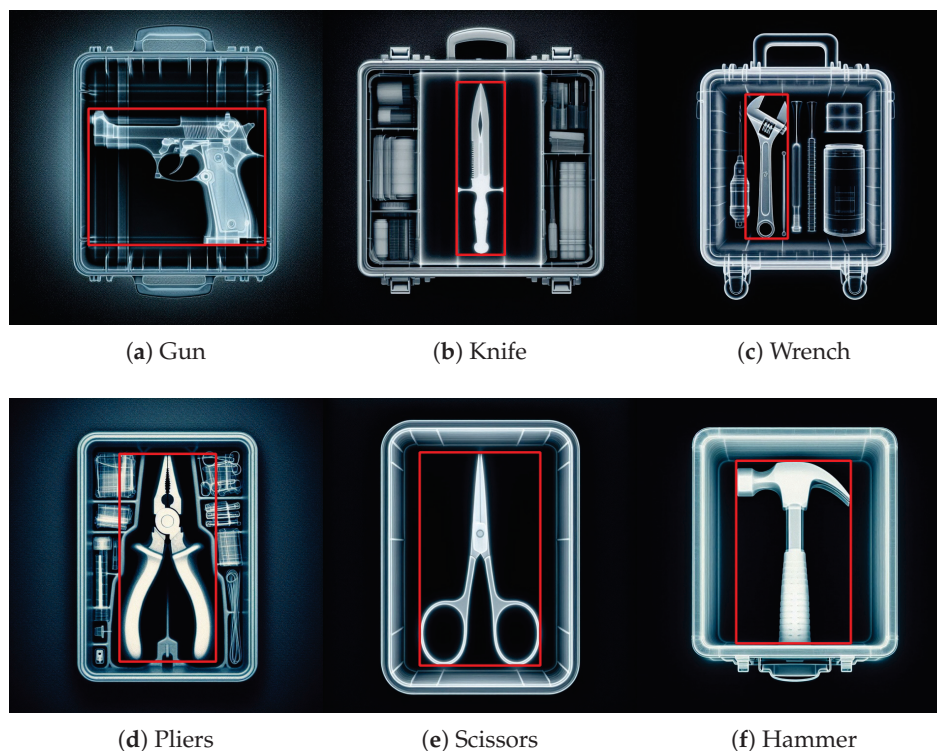
Figure 3. Examples of Gen AI X-ray images for prohibited items that we created, where the red boxes indicate the prohibited items that have been labeled.
