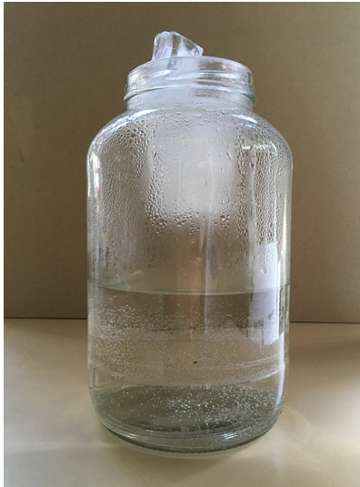
FIG. 3.11 Demonstration of precipitation.
