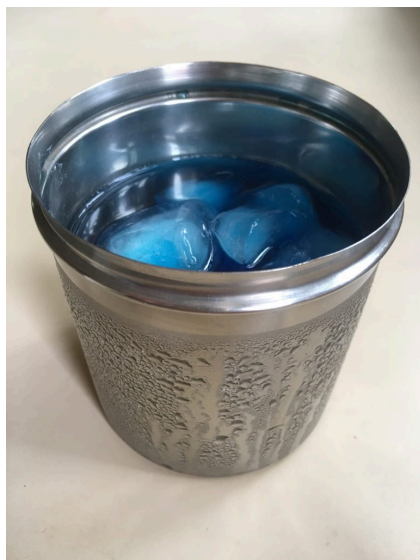
FIG. 3.10 Demonstration of condensation.
