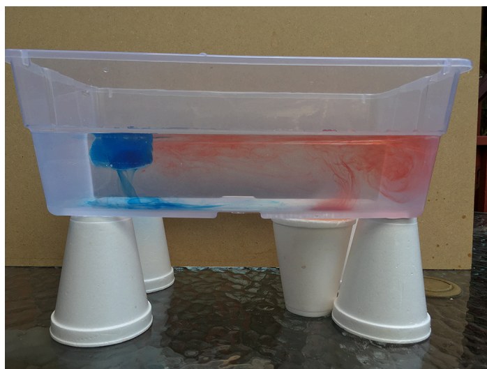
FIG. 3.14 Demonstration of convection currents.
