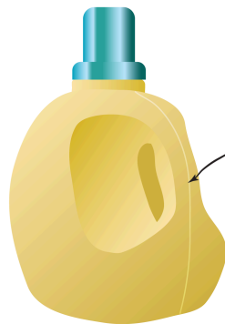
PARTING LINES ON INJECTION MOLDED PLASTICS
