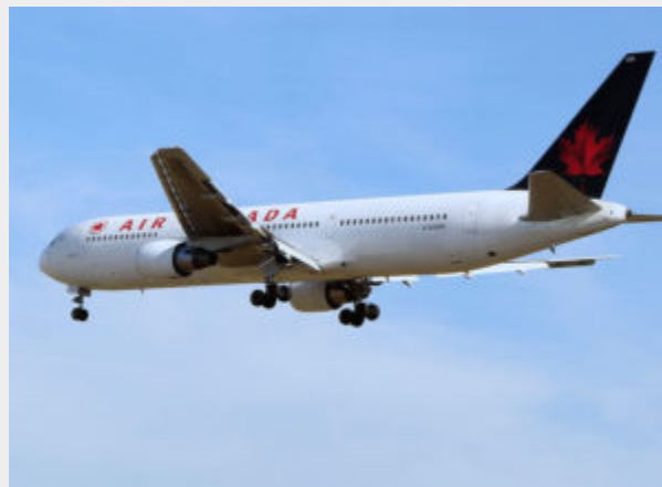
Figure 2.2 “The Gimli Glider.” The Gimli Glider is the Boeing 767 that ran out of fuel and glided to safety at Gimli Airport. The aircraft ran out of fuel because of confusion over the units used to express the amount of fuel.
