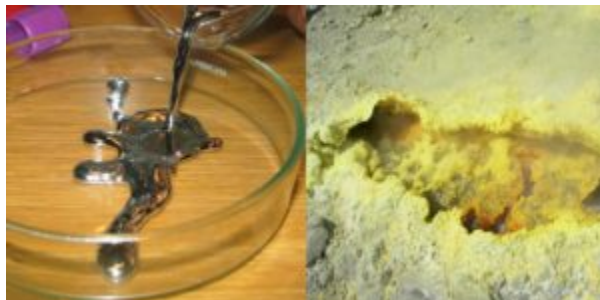
Figure 1.5 “Semimetals.” On the left is some elemental mercury, the only metal that exists as a liquid at room temperature. It has all the other expected properties of a metal. On the right, elemental sulfur is a yellow nonmetal that usually is found as a powder.
