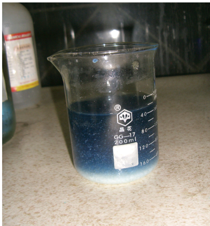
Figure 4.2 “Double-Replacement Reactions.” Some double-replacement reactions are obvious because you can see a solid precipitate coming out of the solution.
