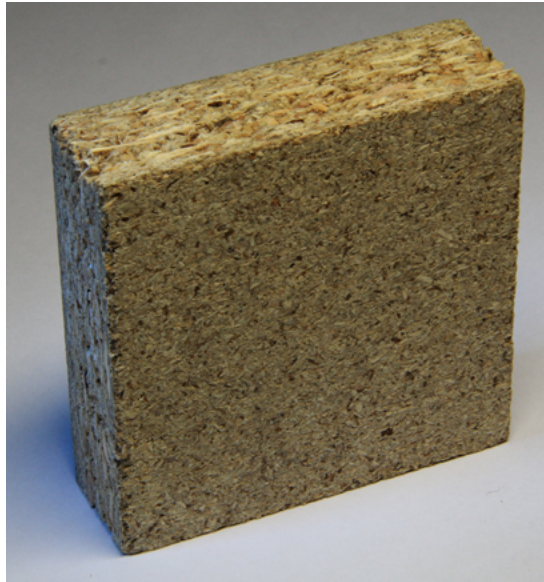
Fig.07/39 Shredded wood waste is held together by formaldehyde resin to manufacture particle boards.
