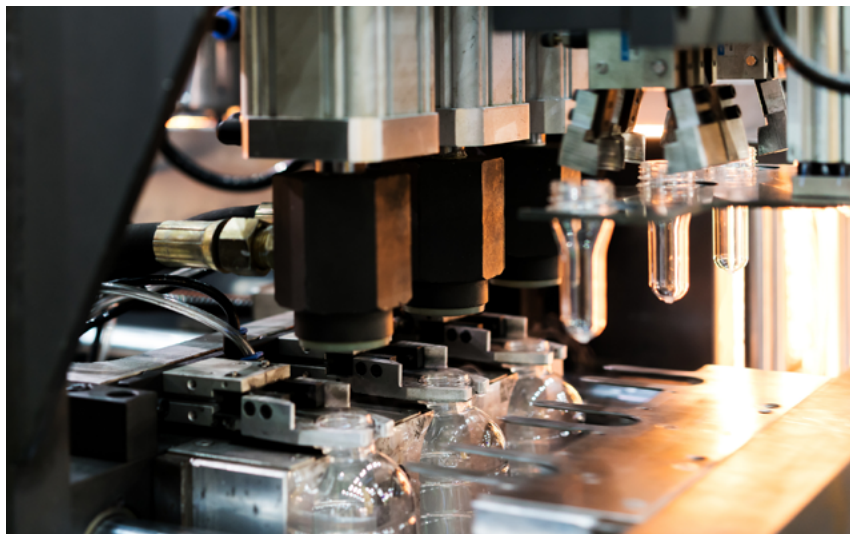
Fig.11/26 In blow molding, the PET billet is heated, and after they are placed within the mold air is pushed in to expand the object into the shape of the mold.
