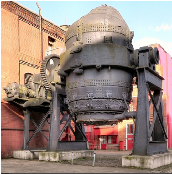
Fig.10/14 The original Bessemer converter design was a huge improvement over blast furnaces.
