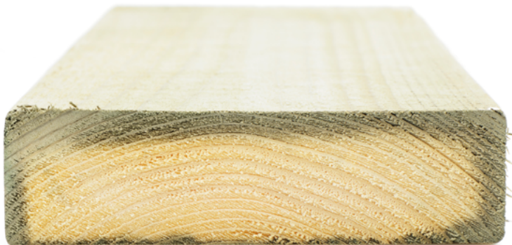
Fig.07/31 The preservative use in the pressure treatment provides significant protection but harms the structural integrity of the lumber.
