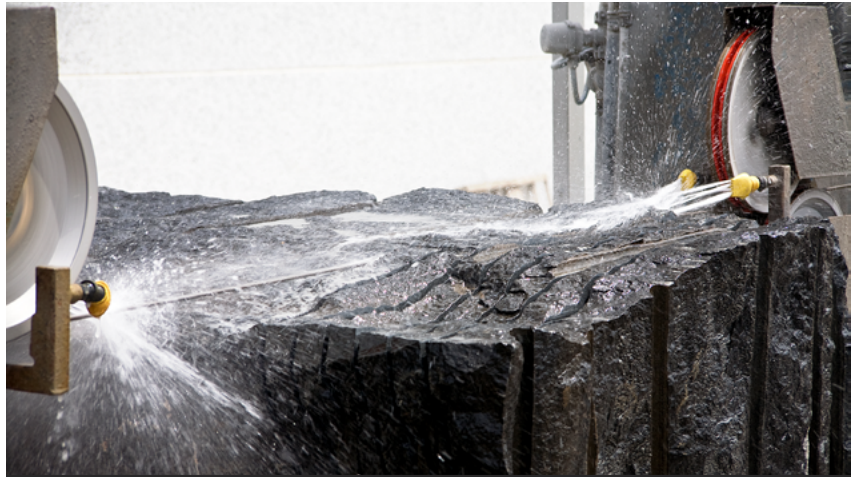
Fig.06/18 The diamond wire needs to be constantly sprayed water to provide lubrication and manage heat build-up.
