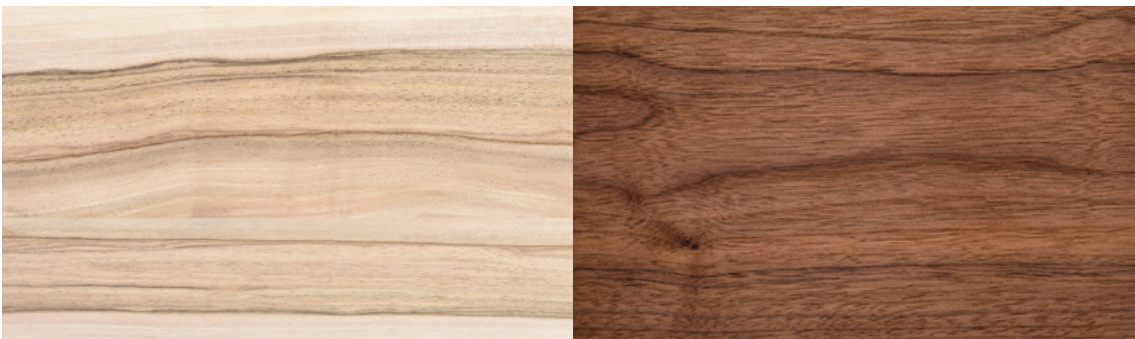
Fig.07/12 The color difference between Walnut sapwood (left) and heartwood (right) is dramatic.
