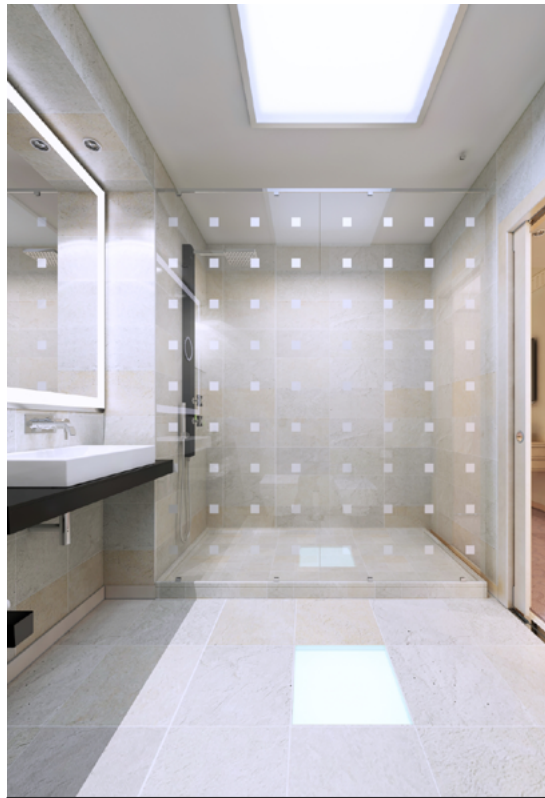
Fig.08/15 Safety squares improve visibility of glass panels, useful where occupant impact is a concern.
