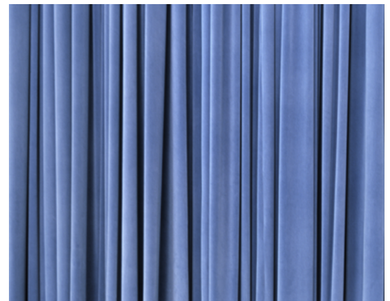
Fig.03/22 A thick velour curtain with deep pleats can provide some acoustic absorption, mostly at the high end of the sonic spectrum.
