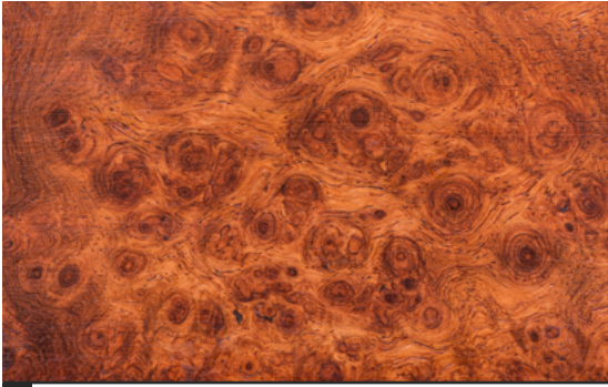
Fig.07/04 Despite being a growth anomaly, burls have highly desirable visual character and are expensive.
