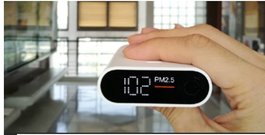
Fig.03/09 A simple particulate meter for residential use.
