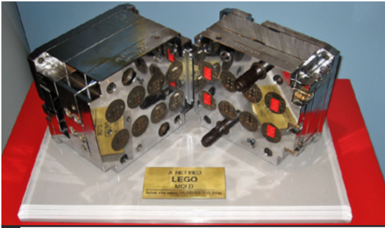
Fig.11/25 A retired Lego injection mold.
