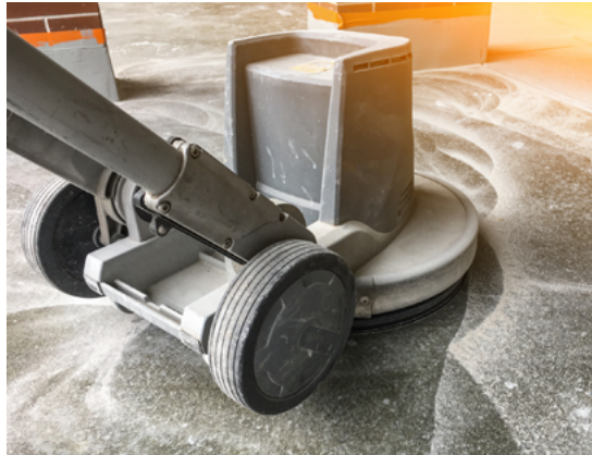
Fig.06/07 Concrete polishers, or floor grinders, feature rotating abraders underneath.
