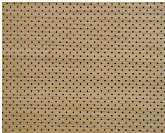
Fig.03/21 Wood can be perforated to achieve acoustic semi-transparency. Without perforations it can only reflect sound waves.
