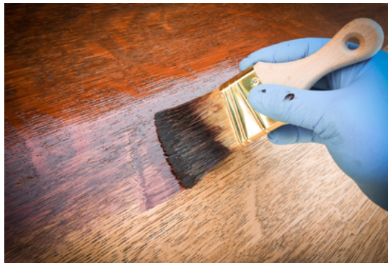
Fig.07/33 Stains can alter wood's look to such an extent that identifying species requires careful inspection.
