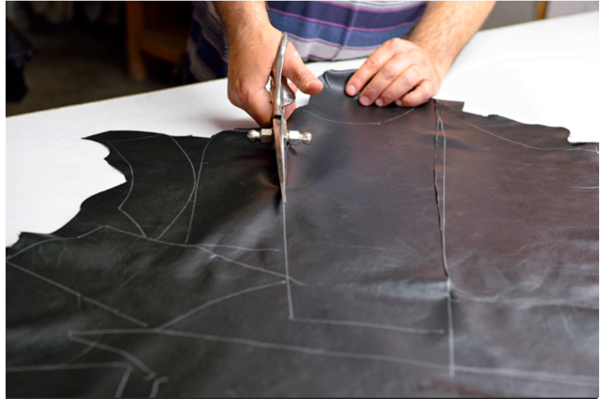
Fig.09/22 The required leather pieces are outlined in a way to keep desired patterns and leave out defects, while using the hide as efficiently as possible.
