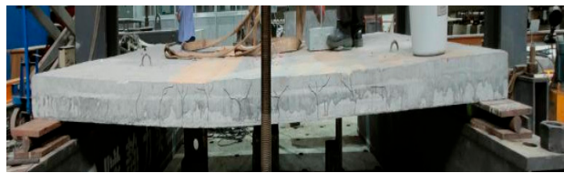
(b) Crack distribution on slab side
