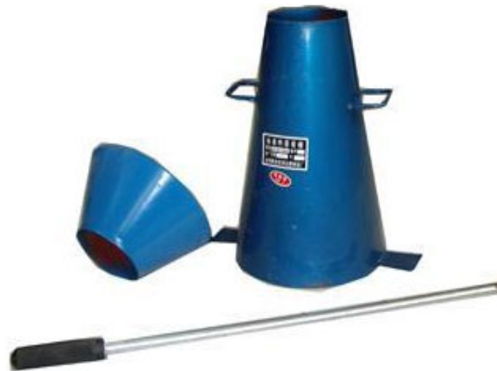
Figure 10. Slump Test Device.
