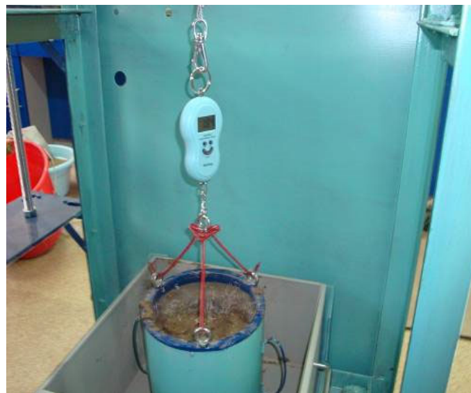
Figure 9. Design of Adhesion Resistance Test Device.
