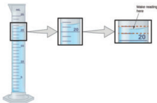
Figure 1 To measure the volume of liquid in this graduated cylinder, you must mentally subdivide the distance between the 21 and 22 mL marks into tenths of a milliliter, and then make a reading (estimate) at the bottom of the meniscus.
