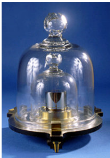
Figure 2 This replica prototype kilogram is housed at the National Institute of Standards and Technology (NIST) in Maryland. (credit: National Institutes of Standards and Technology)
