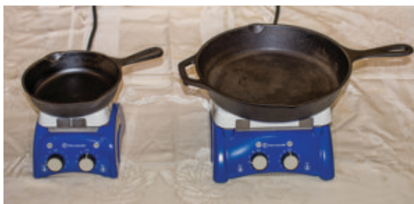
Figure 7 Due to its larger mass, a large frying pan has a larger heat capacity than a small frying pan. Because they are made of the same material, both frying pans have the same specific heat. (credit: Mark Blaser)
