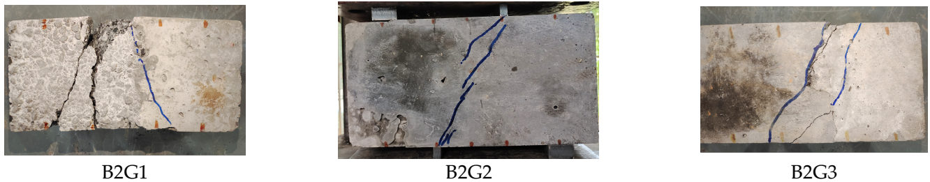
Figure 7. Shear damage with different rebar diameters.
