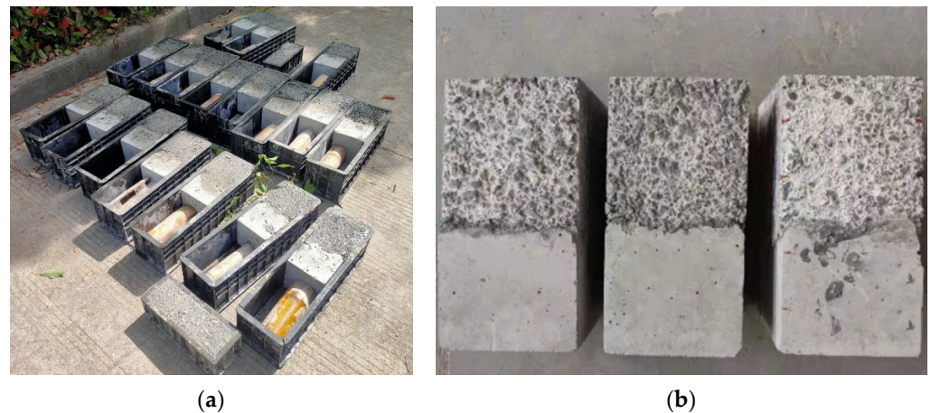
Figure 3. New and old concrete specimens. (a) After pouring. (b) After demolding.
