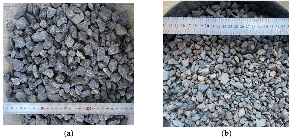
Figure 1. Coarse aggregates. (a) Ordinary crushed stone. (b) Ceramsite pellets.
