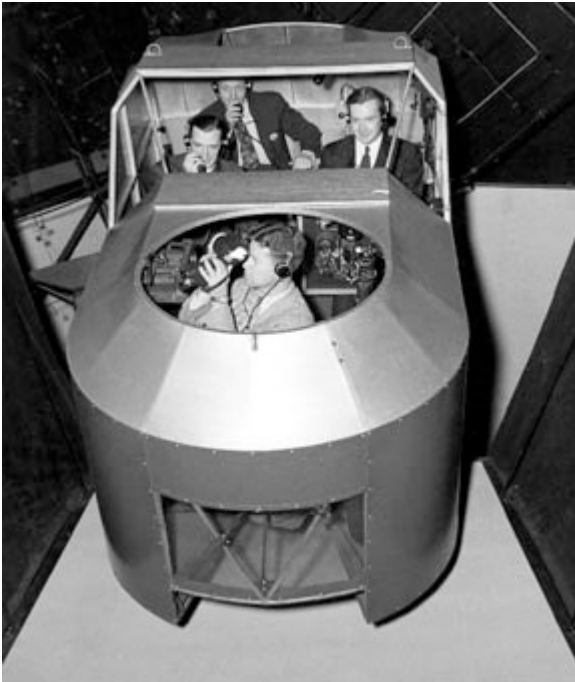
The Link Celestial Navigation System?. You can see the “cockpit” with the navigator and pilot trainees shown above. They were situated right under the projection dome.
