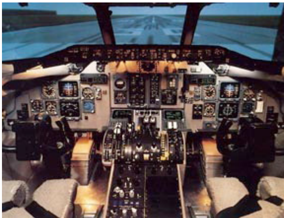
The visual component of the simulator generated images that were presented to the training pilot on display devices mounted inside the physical simulator.
