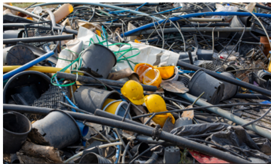
Fig.11/03 A heap of PVC waste including rigid and flexible components, waiting for separation.
