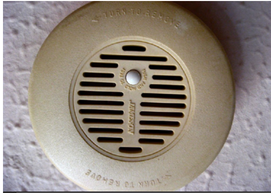
Fig.11/10 Without stabilizers, PVC yellows over time. A useful quality to indicate component age.
