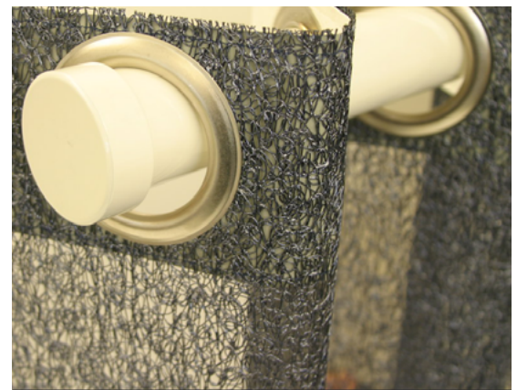
Fig.11/06 Thermoplastic Polyurethane (TPU) drape, TPU is the thermoplastic version of the widely employed thermoset plastic polyurethane (PU).
