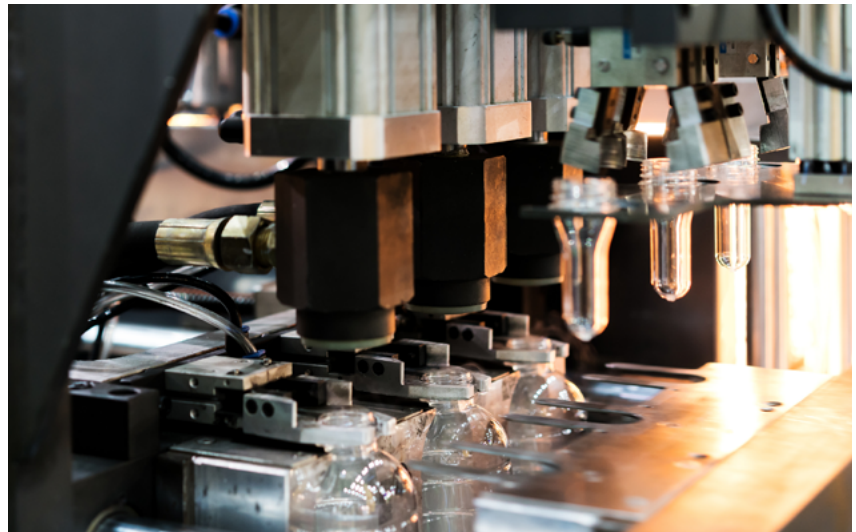
Fig.11/26 In blow molding, the PET billet is heated, and after they are placed within the mold air is pushed in to expand the object into the shape of the mold.
