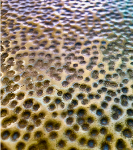
Fig.10/01 The malleability of metals enables the creation of hand-made textures such as hammered bronze.
