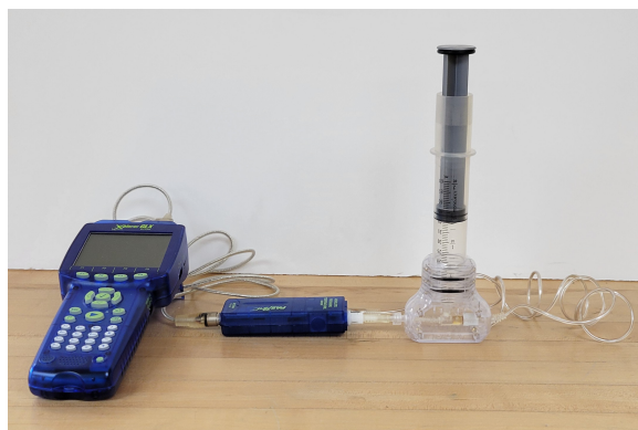
Figure 26.1: Ideal Gas Law Apparatus
