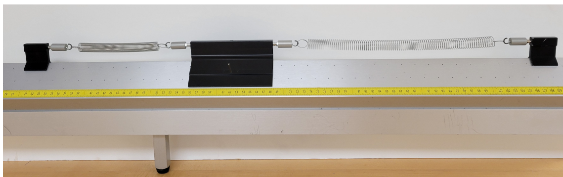
Figure 21.6: Cart Connected to Two Springs on an Air Track
