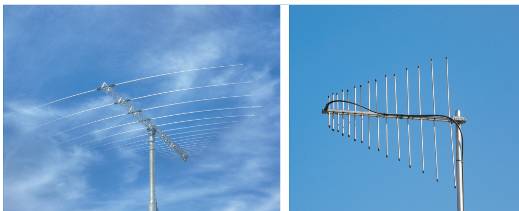
FIGURE 63 Antennas for horizontally and vertically polarized electromagnetic waves (© Martin Abegglen, K. Krallis).
