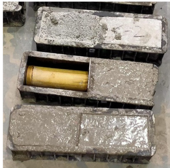
Figure 1. Bonding method of new and old concrete.
