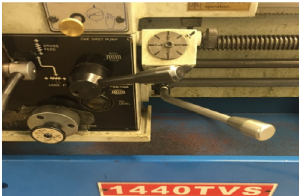
Figure 11: On/Off Lever and Half Nut
