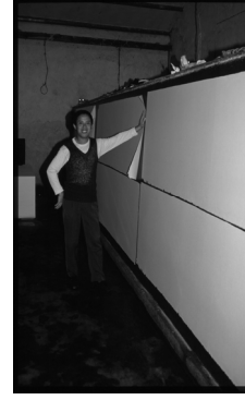
Figure 18: Drying paper on a moderately hot metal wall, Jingxian, Anhui.
