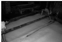
Figure 14: Forming a sheet of calligraphy paper, two-man, three-direction flow method, Jiajiang, Sichuan.
