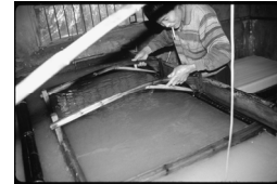
Figure 12: Forming a sheet of calligraphy paper ( shuhuazhi ), single-dip method, Fuyang, Zhejiang.
