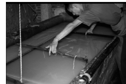
Figure 15: Forming a sheet of calligraphy paper, one-man, three-direction flow method, Jiajiang, Sichuan.
