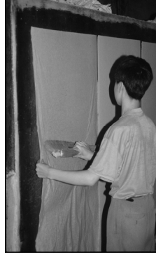
Figure 17: Drying paper on a very hot metal wall, Fuyang, Zhejiang.
