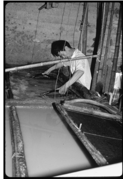
Figure 11: Forming a sheet of bamboo paper ( zhuzizhi ), single-dip method, Fuyang, Zhejiang.
