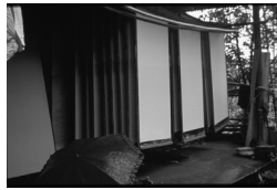
Figure 20: Sheets of paper drying on large wooden planks hanging under the eaves of a papermaker's home, Jiajiang, Sichuan.
