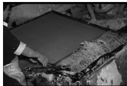
Figure 13: Forming a sheet of Korean-style paper ( Gaolizhi ), two-direction flow, Qian'an, Hebei.
