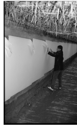
Figure 21: Sheets of Korean-style paper drying on plaster-covered walls built outdoors, Qian'an, Hebei.
