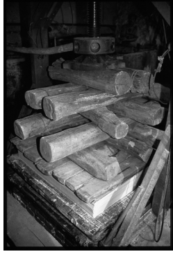
Figure 16: Pressing a post of Korean-style paper, Qian'an, Hebei.
