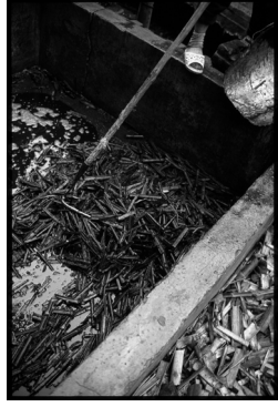
Figure 7: Retting bamboo fibers in a large concrete vat, Jiajiang, Sichuan.
