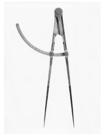
fig. 2.20 Late seventeenth-century wing dividers. From Maya Hambly, Drawing Instruments, 1580–1980 (Sotheby's Publications, 1988), p. 26, fig. 60.
