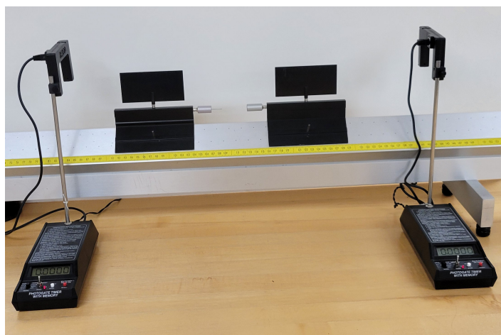
Figure 16.3: Completely Inelastic Collision Between Carts On An Air Track
