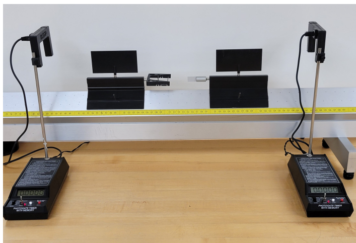
Figure 16.1: Perfectly Elastic Collision Between Carts On An Air Track
