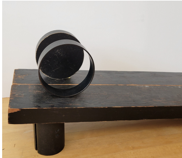
Figure 19.1: Ring and Disk Roll Down an Incline
