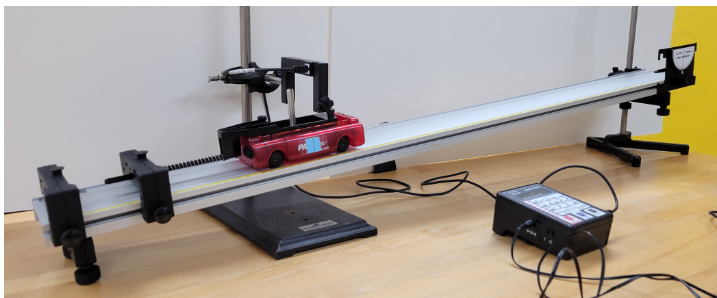
Figure 14.4: Set-Up of Dynamics System to Verify the Conservation of Mechanical Energy
