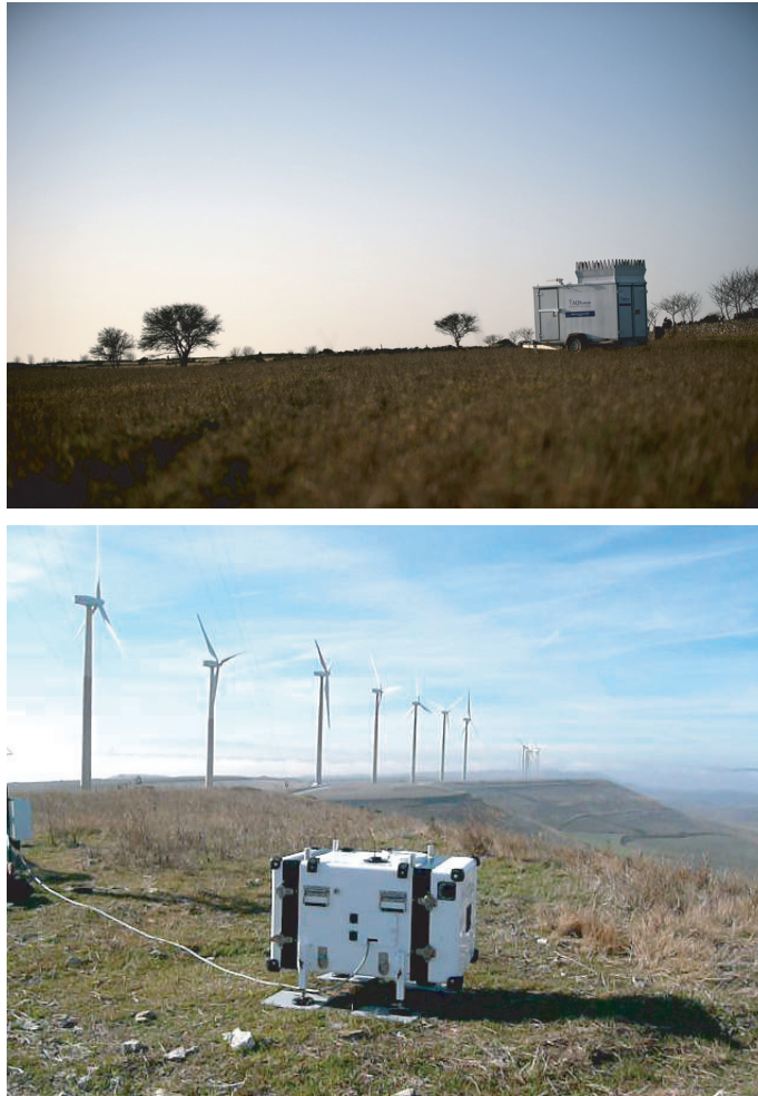
FIGURE 266 Two wind measuring systems: a sodar system and a lidar system (© AQSystems, Leosphere).
