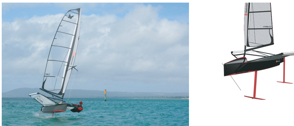
FIGURE 258 The moth sailing class: a 30 kg boat that sails above the water using hydrofoils , i.e., underwater wings (© Bladerider International).
