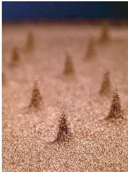
FIGURE 289 Oscillons formed by shaken bronze balls; horizontal size is about 2 cm (© Paul Umbanhowar)
