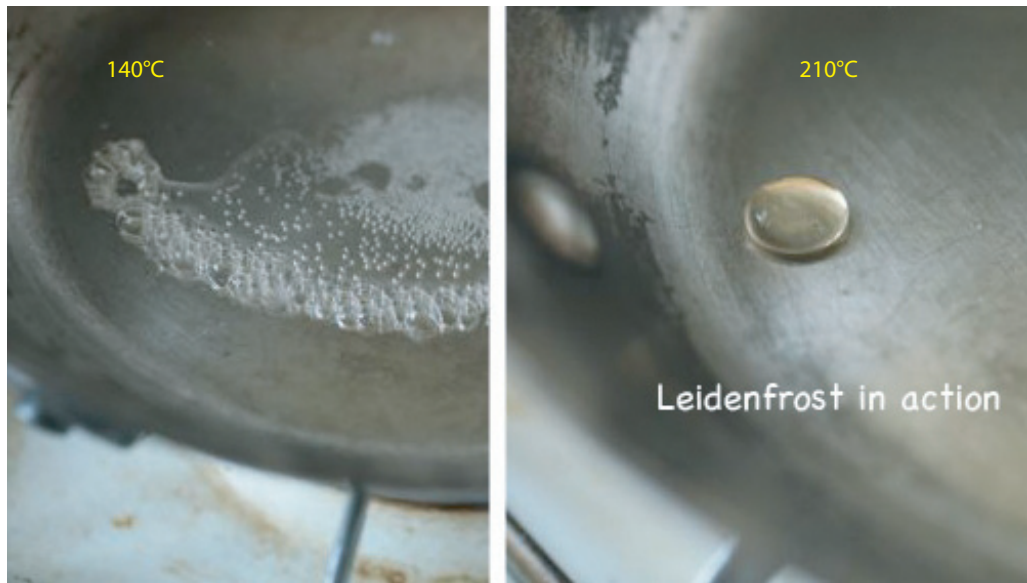
FIGURE 267 A water droplet on a pan: an example of the Leidenfrost effect (© Kenji Lopez-Alt).
