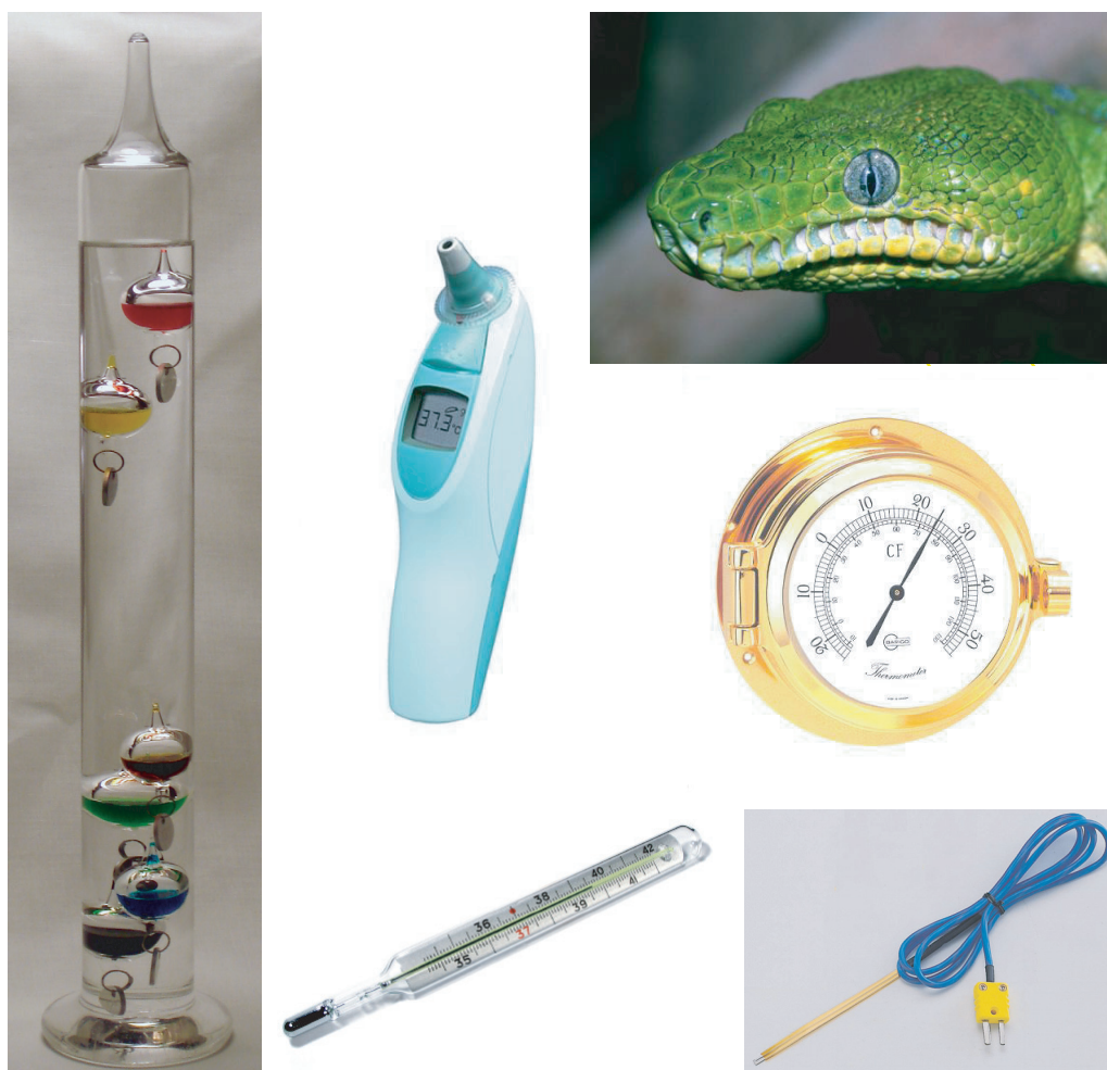
FIGURE 275 Thermometers: a Galilean thermometer (left), the row of infrared sensors in the jaw of the emerald tree boa Corallus caninus , an infrared thermometer to measure body temperature in the ear, a nautical thermometer using a bimetal, a mercury thermometer, and a thermocouple that is attached to a voltmeter for read-out (© Wikimedia, Ron Marcus, Braun GmbH, Universum, Wikimedia, Thermodevices).
