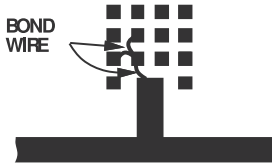
Figure 3-16: Open-circuited stub with variable length realized using wire bonding from the fixed stub to one of the bond pads. The bond pads are on the same layer as the strip metal layer and bonding to them extends the length of the open-circuited stub.
