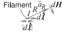
Figure 1-3: Diagram illustrating the Biot-Savart law. The law relates a static filament of current to the incremental H field at a distance.
