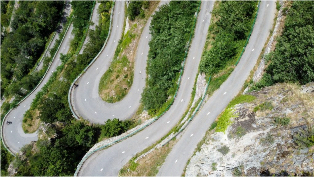
Figure 1: Horizontal profile (top view) of a road with significant horizontal curvature. Landscape, Aerial View, Mountain Road by Freddy Dendoktoor under (CC0 1.0)
