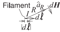
Figure 1-3: Diagram illustrating the Biot-Savart law. The law relates a static filament of current to the incremental H field at a distance.
