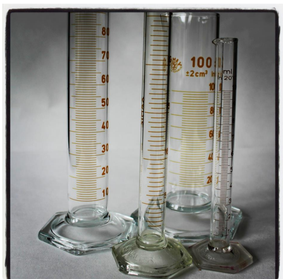
Figure 3.5: Graduated Cylinder: " Laboratory Equipment - Graduated Cylinder " by eltpics is licensed under CC BY-NC 2.0 .
