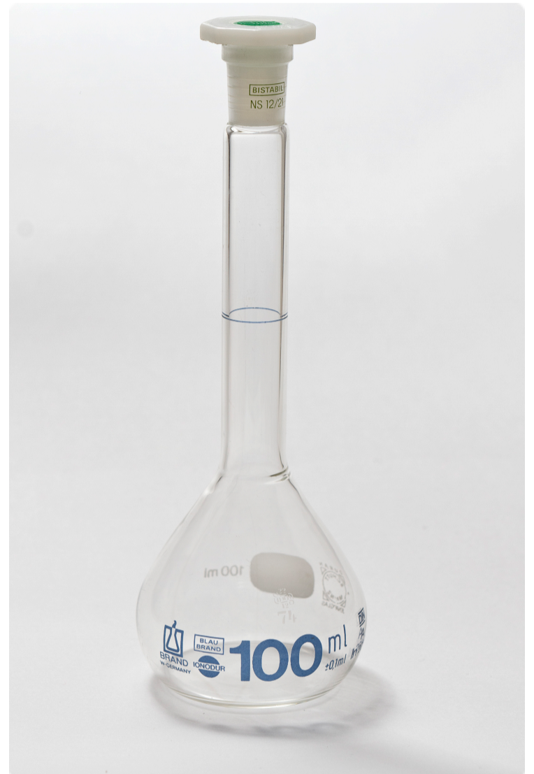
Figure 3.9: Volumetric Flask: " File:Brand volumetric flask 100ml.jpg " by Lucasbosch is licensed under CC BY-SA 3.0 .
