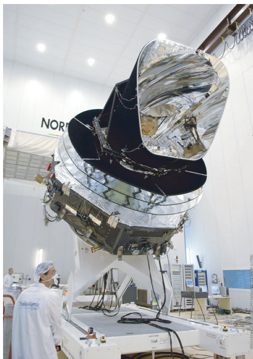
FIGURE 97 Top: the XMM-Newton satellite and its high-precision, onion-like mirrors that produced an X-ray map of the night sky. Bottom: the Planck satellite and its golden-plated microwave antennas that produced a high-resolution map of the cosmic background radiation (© ESA).
