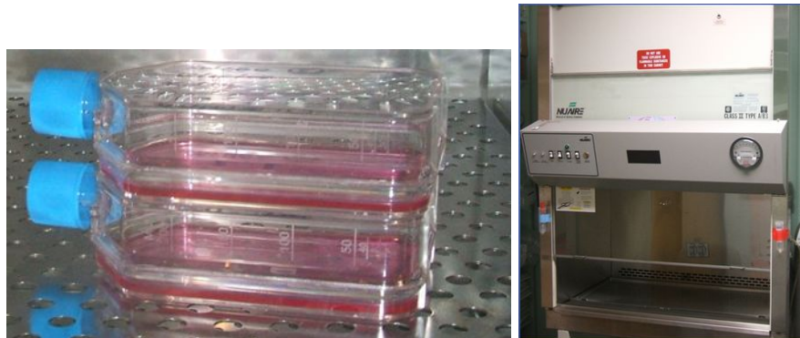
Figure 1.32 Flask containing media and cells (left); biosafety cabinet (cell culture hood, right)
