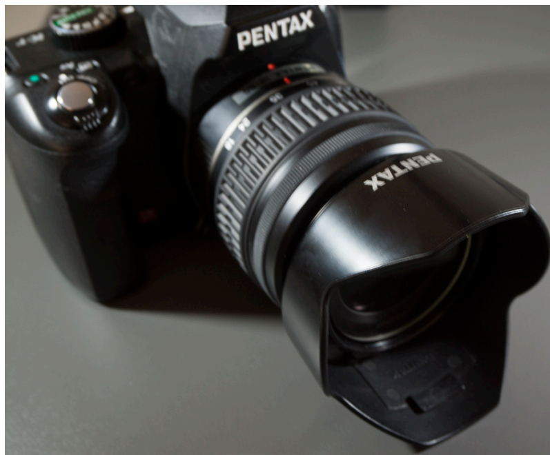
Figure 14-14. A lens hood reduces reflected glare onto the lens, which increases the contrast of photos and avoids artifacts from stray light.
