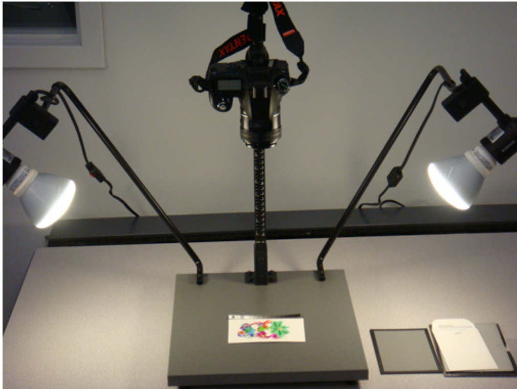
Figure 14-10. A copy stand is useful for photographing flat objects. Two lights at 45° angles help reduce glare from the subject's surface.
