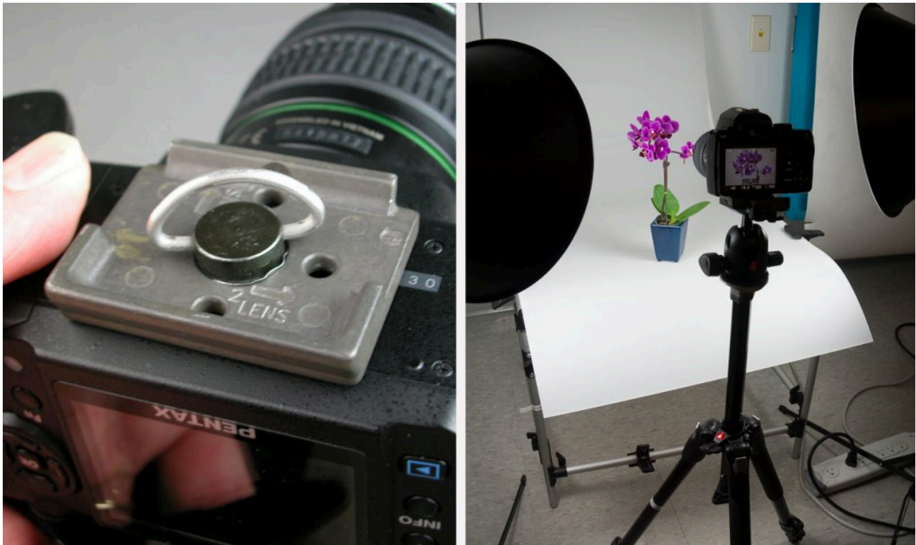
Figure 14-5. Quick-release tripod mount includes a plate that screws into the camera mount and then clips onto the tripod, allowing for rapid on-and-off operation.
