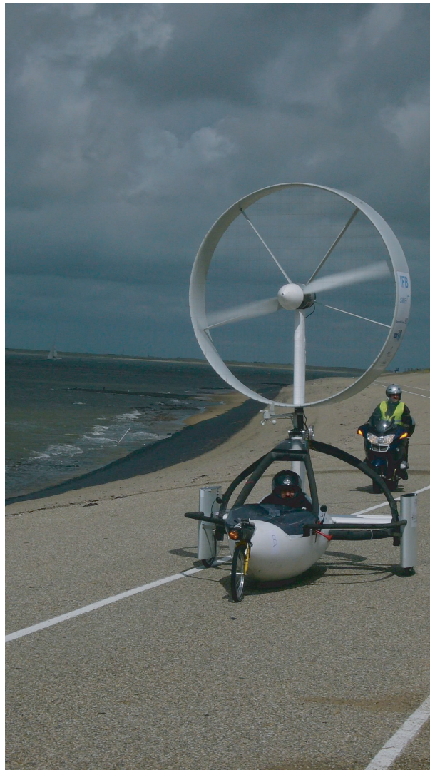
FIGURE 327 A way to ride head-on against the wind using wind power (© Tobias Klaus).
