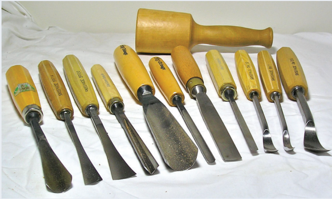
Figure 2.23 | A selection of woodcarving gouges, chisels, and a mallet
