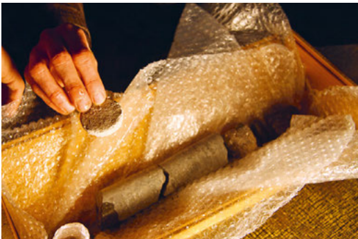
Fig. 1.6: For several material samples (a core drill hole, painting and plaster samples from the exterior wall, material samples from the wooden beams and the filling of the ceiling density)
