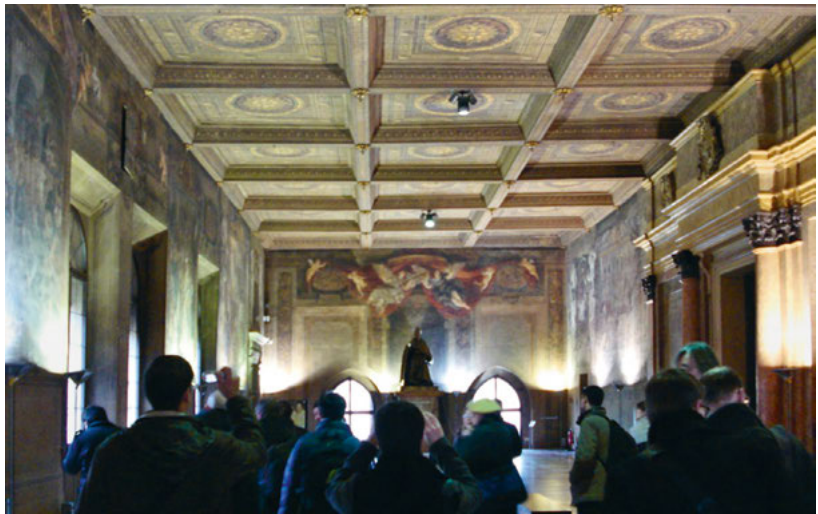
Fig. 5.50: Pre-3ENCULT: the lighting system produces high inhomogeneities and glare.
