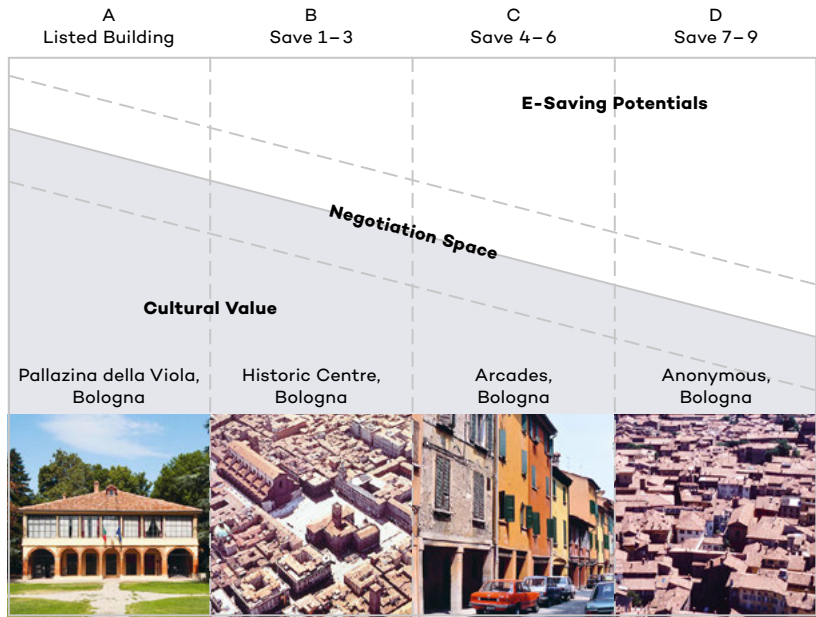
Fig. 4.4: Four classes of cultural value based on the SAVE categories 1–9 with different options for saving energy.
