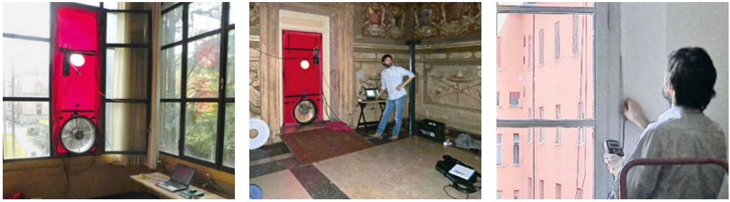
Fig. 3.22: BDT equipment and fan mounted on historic window (left), BDT testing with fan installed in door (middle), BDT test: checking air infiltration with a hot-wire anemometer (right)
