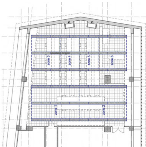
Fig. 7.7: Redistribution of the luminaires in the physics laboratory
