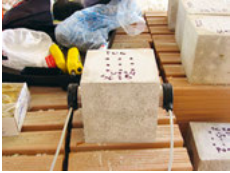
Fig. 3.21: Sonic test on masonry wall (top), ultrasound testing of a concrete block (bottom)
