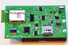
Fig. 6.17: Wispes W24TH node sensor specifics: Temperature: 14-bit codification, 0.01°C resolution, \pm 0.3 accuracy, -40 to 125°C operative range Humidity: 12-bit codification, 0.04% RH resolution, \pm 2\% RH accuracy, 0 to 100% RH operative range Ambient light sensor: 0.23 to 100,000 lux operative range, \pm 15\% accuracy
